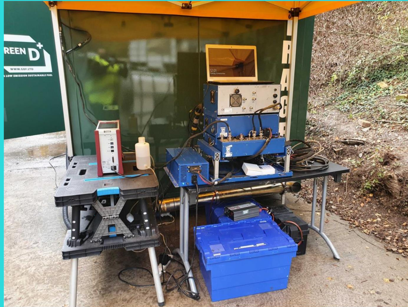
Figure 1 - PEMS setup for static generator testing
