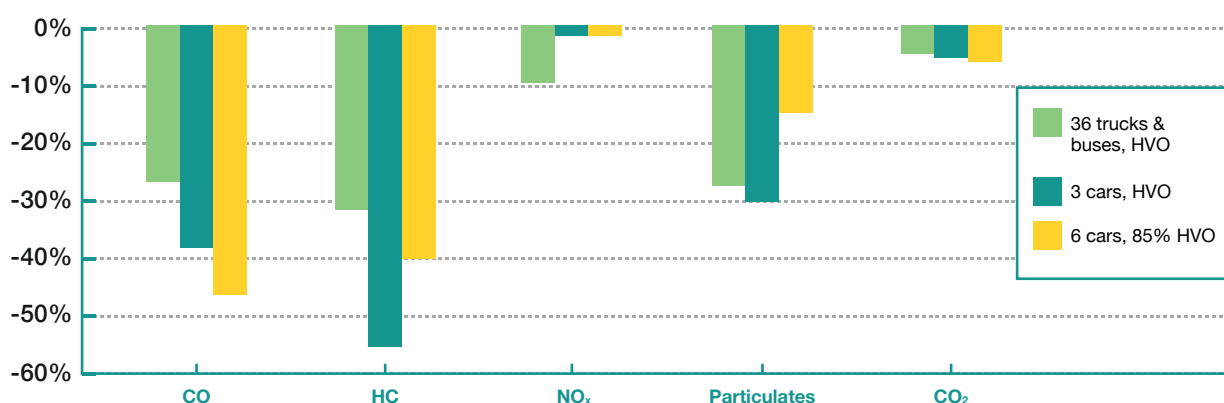
Figure five: Average effect of neat and almost neat (85%) Neste Renewable Diesel (HVO) on tailpipe emissions EURO II and EURO VI vehicles compared to a Sulphur-free EN 590 diesel fuel
